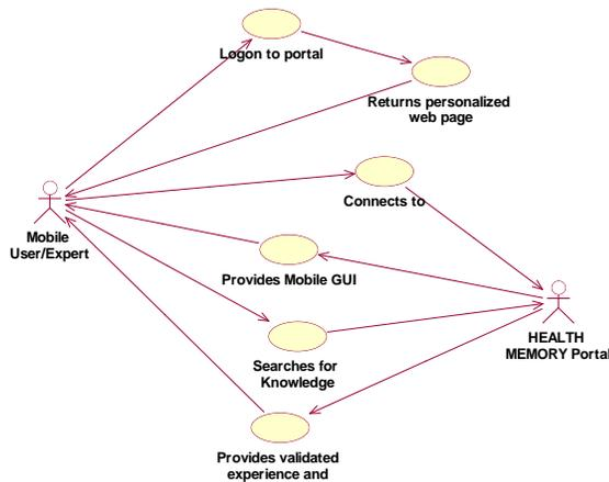
Fig. 3. Use case scenario for mobile platform
